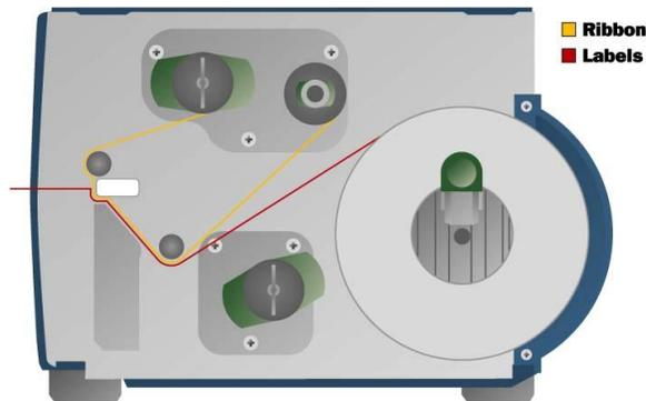
The resulting image is stable and unaffected by heat or exposure to light. Thermal transfer printers are just as versatile as direct thermal printers with the additional advantage that plain paper labels can be used. Depending on the combination of labels and ribbon the image is suitable for
