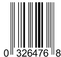
Is a fixed length, 6 digit numeric code. It is a compressed code ideal for use on small packages. It is also known as the zero suppression version of UPC-A. It allows manufactures to encode a limited number of 12 digit codes in six digits.
