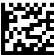
Is a two-dimensional variable length symbology capable of encoding ASCII characters. Each code has a unique perimeter pattern that is used to determine the orientation. Two of the outside rows are solid, forming the letter 'L' and the opposite two sides use alternating black and white patterns which help synchronize the decoding process. Up to 2334 characters can be encoded.
