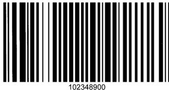
A subset of Code 128, using a special Code 128 character creates the EAN-128. The Function Code 1 (FNC 1) when encoded immediately after the start character has been reserved to indicate that the data follow conforms to the EAN/UPC structure. The ANA, EAN and UCC have reserved its usage.
