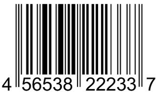
The Uniform Product Code (UPC) has been successfully used in the retail industry in the United States and Canada since 1973. This is a coding system as well as a symbology. It is designed to uniquely identify a product and its manufacturer. The UPC-A code is a 12 digit numeric code. The first six digits represent the manufacturer, the next five digits are a unique product identifier and the twelfth is a check digit. The first six digits are allocated by the UCC (Uniform Code Council).
