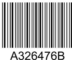
Codabar is a numeric only symbology. It has 4 different start and stop characters that can be used to identify different types of data. Using a correct combination of these start/stop characters it is possible to read two adjacent bar codes simultaneously
