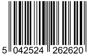
The EAN (European Article Numbering) system has two common versions. The EAN-13 and EAN-8 encoding 13 and 8 numeric digits respectively. The EAN symbology was developed for one requirement: to enable grocery products to be scanned at the Point of Sale. The symbol contains numeric data only.
