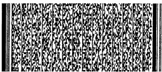
The most common 2-D stacked code today is the PDF417. This is a variable length symbol. Each character consists of 4 bars and 4 spaces in a 17-module length. This is a (17,4) structure-giving rise to the symbology name. There are 929 character values in each of three different sets. A given row uses one character set whilst the two adjacent rows use different sets.
