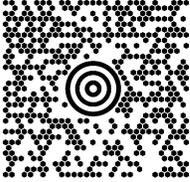
Developed by United Parcel Service for the automatic sortation and tracking of packages. It is a fixed length alphanumeric symbology composed of an array of interlocking hexagons surrounding a circle pattern. 144 characters can be encoded.
